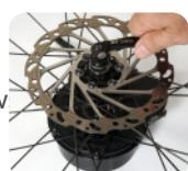
2. Reassemble the quick release and tighten
