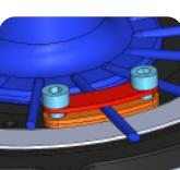
3. Loosen the original locked M3x8mm (C2) screws and put one more clamp on the spoke (as illustrated)
