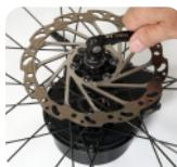
4. Reassemble the quick release to the center hole of the wheel and tighten it down with the mounting component (D).
