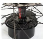
3. Place the right-center axis of the hub onto the dynamo F12W-PRO (A).
