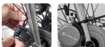
10. Tighten the shockproof rubber (a1)
