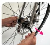
1. Remove quick release and front wheel.
