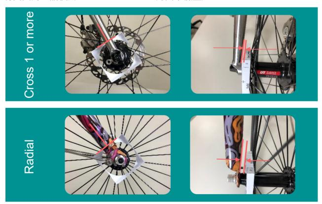
7. If the measuring tool doesn't touch the fork, you are ready to install the F12W-PRO! 如果檢查工具沒有觸碰到您的前叉,您將有足夠的空間安裝 F12W-PRO!
